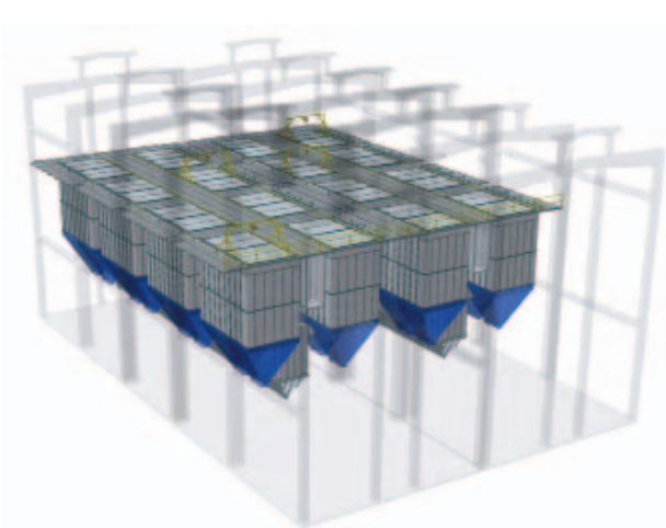
Reverse air dust collector converted to pulse-jet.
